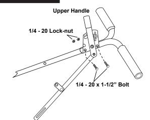
**9.** Insert (2) 1/4-20 x 1<sup>1</sup>/<sub>2</sub>" Hex Bolt through Gauge and Linkage Assembly, then through the Upper Handle, Handle Shaft, Upper Handle and secure with (2) 1/4-20 Locknuts as shown at the right.
