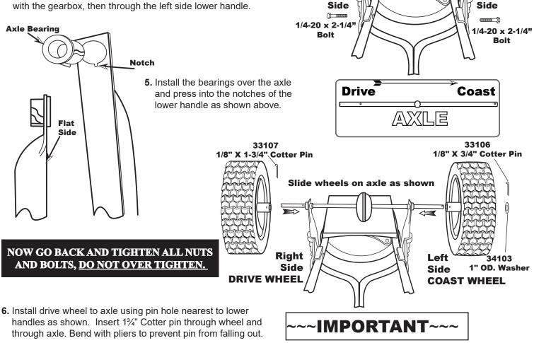
Install coast wheel to axle using outside pin hole. As shown, add the flat washer, and insert <sup>3</sup>/<sub>4</sub>" Cotter pin through axle (not thru the wheel). Bend with pliers to prevent pin from falling out.
