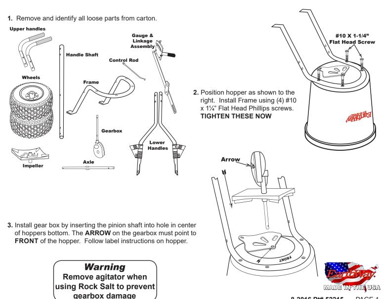
**4.** Install lower handles onto Frame and secure with ¼-20 x 2¼" bolt through hole in Frame Braces and through the hole in frame install locknut.
