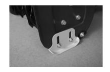
Adjustment of the skid shoes sets the height above the ground at which the auger shave plate operates.
