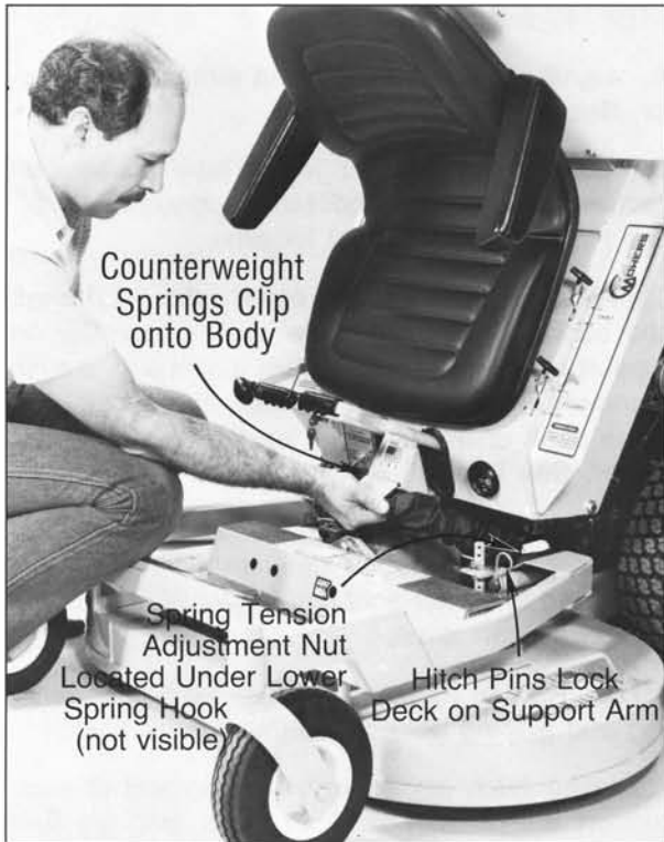
PHOTO 3-7 Deck Counterweight Spring Installation
