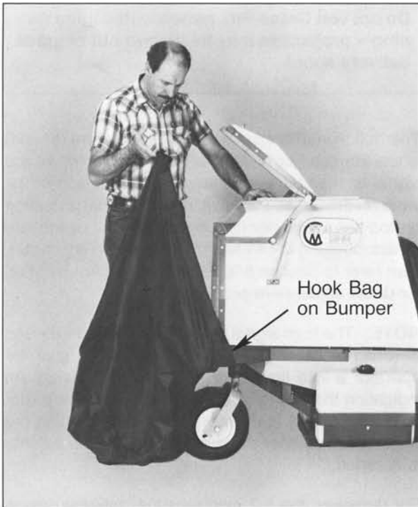
PHOTO 4-6 Positioning Dump Bag on 6.7 Bushel Catcher
