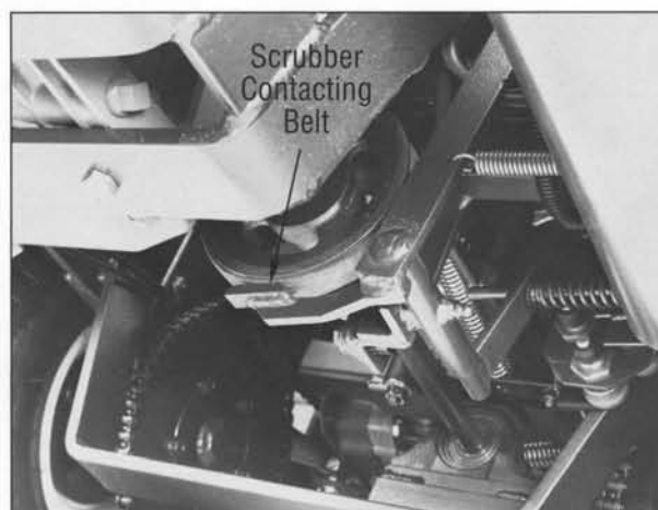
PHOTO 5-23 Scrubber Brake Adjustment on Standard SD Model
