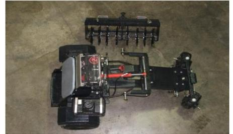
Once the traction unit is free of any attachments (in the under carriage area), slide the Snow Blade under the unit with the frame Draw Pins facing forward. Rest Draw Pins on front tires (*pictured below*) and re-position yourself in the front of the traction unit. Lift Draw Pin up into Front Frame Bracket and lock with Lynch Pins (*pictured below*)
