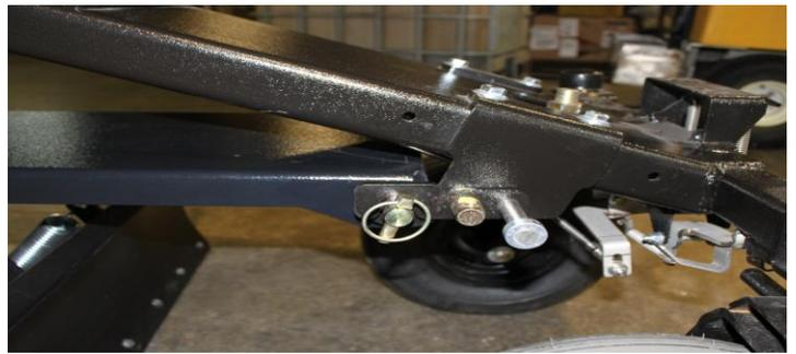
(Snow Blade locked into the Aerator Front Frame)
