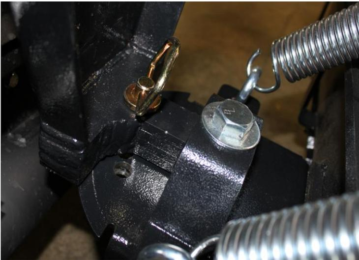
(adjustment pin and pivot to angle blade)
