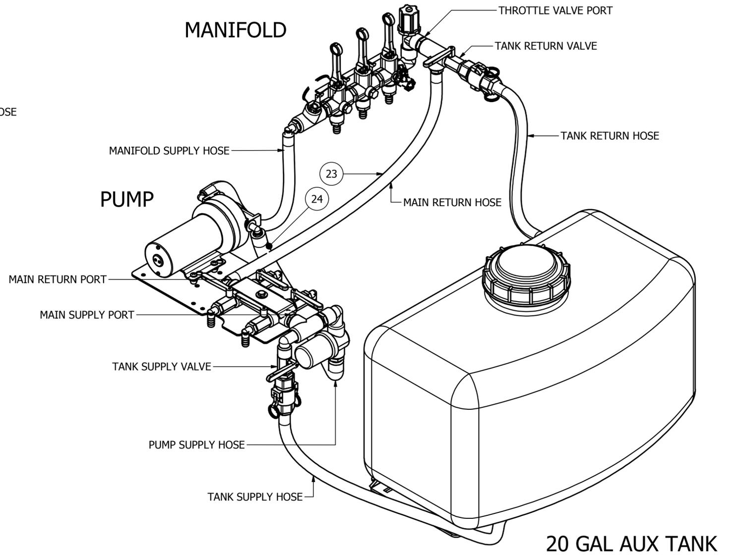
\*THE LIQUID MANIFOLD AND PUMP ASSEMBLIES ARE PART OF THE SPRAYER AND NOT INCLUDED WITH THE 20 GAL AUX ATTACHMENT.
