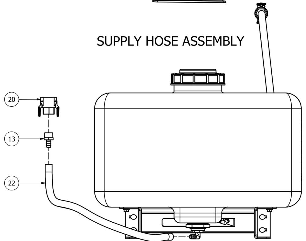
NOTES: 1. APPLY SILICONE SPRAY TO HOSE ENDS BEFORE ATTACHING.
