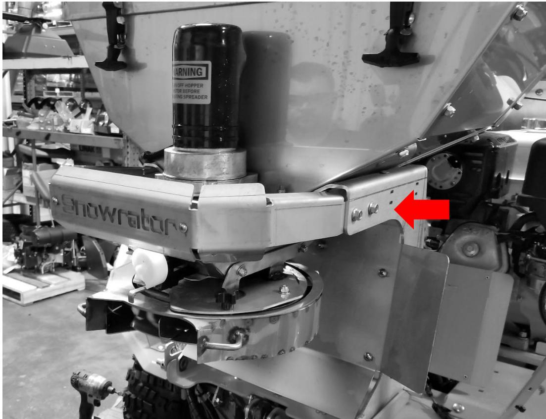
ROTATE SHAFT TO GAIN ACCESS TO BOTTOM SET SCREW IN COLLAR.
