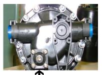
Pressure adjust on pump (Allen Wrench)
