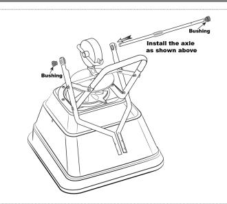
**Step 8:** Install drive wheel onto the axle and align with the cotter pin hole nearest to lower handles as shown. Insert 2" cotter pin through wheel and through axle. Bend with pliers to prevent pin from falling out.
