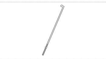
**Step 15:** Install flattened end of control rod in to lever on gauge as shown. Turn to lock in place. Next push lever forward to setting "0". Align control rod with hole in pivot bracket, pull lever backward to insert control rod through hole in pivot bracket. Now install ¼-20 Hex nut on to control rod.
