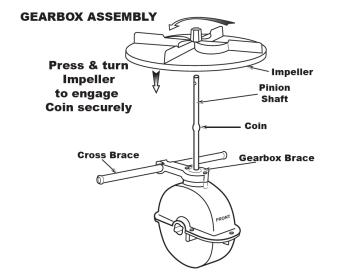
**Step 4:** Install gearbox by inserting the pinion shaft into hole in center of hoppers bottom.
