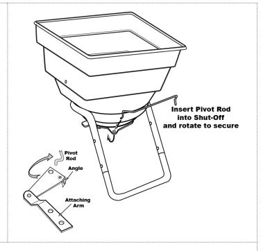
**Step 13:** Install handle shaft to lower handles and pivot & bracket assembly as shown. Using ¼-20 x 2" bolts and locknuts. **TIGHTEN BOLTS AND NUTS NOW**.
