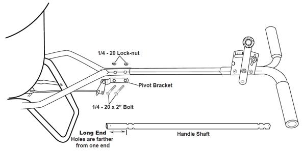
**Step 14:** Install (1) ¼-20 Hex nut (not a locknut) on to control rod as shown.
