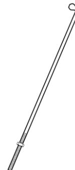
**Step 13:** Install flattened end of control rod in to lever on gauge as shown. Turn to lock in place. Next push lever forward to setting "0". Align control rod with hole in pivot bracket, pull lever backward to insert control rod through hole in pivot bracket. Now install 1/4-20 Hex nut on to control rod.
