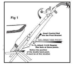
Lever to #30. Next tighten each nut so that they contact the pivot bracket without moving it. Carefully tighten each nut fully so they do not loosen during use. Recheck adjust as outlined in #1 above.
