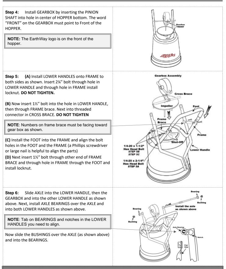
NOW GO BACK AND TIGHTEN ALL NUTS AND BOLTS STARTING WITH FIRST STEP. DO NOT OVER TIGHTEN.
