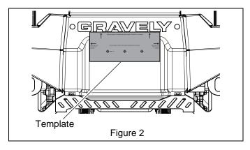
Mark center of three mounting holes with center punch.
