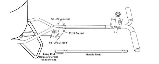
**Step 13:** Install (1) 1/4-20 (M6 X 1) regular nut (not a locknut) on to CONTROL ROD.
