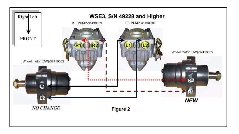
On MMZ & WSZK models serial 49228 and below it is the right side wheel motor when standing in front of unit. The high pressure hose that was originally in the top port of the wheel motor will move to the bottom port and the hose in the bottom port originally will move to the top port of the wheel motor.
