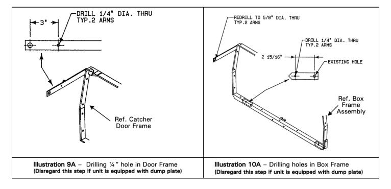
10. Redrill existing door pivot hole in box frame assembly to 5/8", as shown in Illustration 10A. In some cases, a pivot bushing is installed in the frame. Remove this bushing to expose the 5/8" hole. Remove door springs and remove door frame assembly (View 9A) from the catcher box. Drill a 1/4" hole in both door frame assembly arms, as shown in View 9A. Check location of hole by inserting door actuator arms (View 9B) into door arms.
